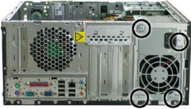
FIGURE 7: Removing the power supply screws
