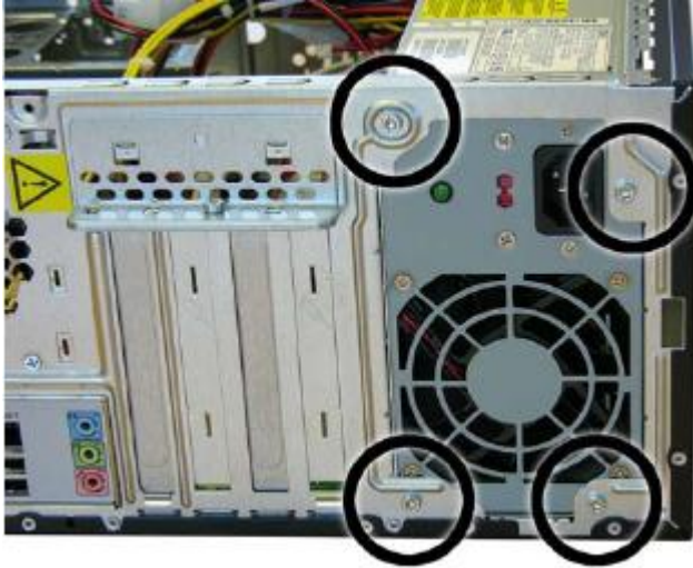
FIGURE 7: Removing the power supply screws
