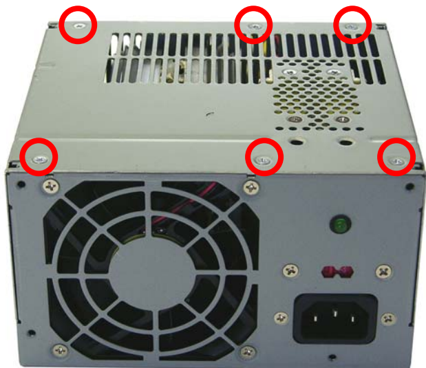
FIGURE 9: POWER SUPPLY : Cover screw locations
