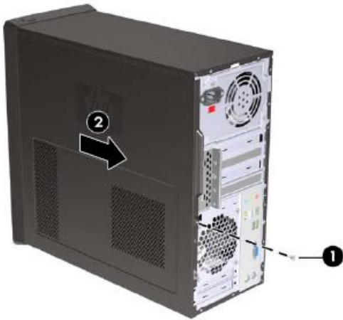
FIGURE 1: Removing the access panel.
