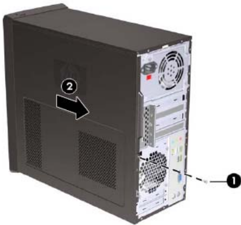
FIGURE 1: Removing the access panel.
