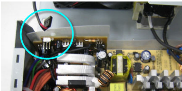
FIGURE 10: Disconnect two control cables
