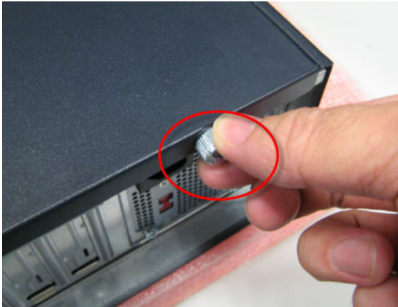
FIGURE 2: Remove the access panel
