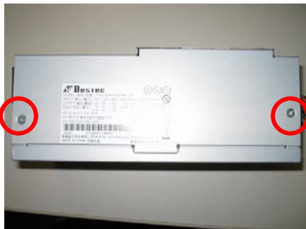
FIGURE 7: Power supply cover screw locations on the top side
