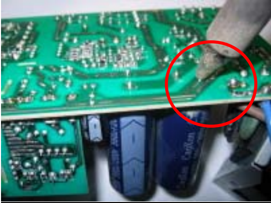
FIGURE 15: Remove the Electrolytic Capacitors
