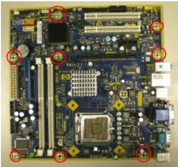
Figure 5: Remove the system board
