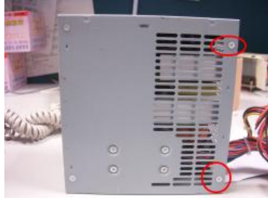
Figure 8: Power supply cover screw locations on the right side
