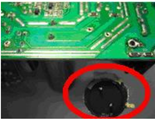
Figure 15 : Remove the Electrolytic Capacitors
