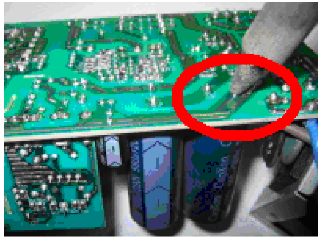
Figure 14 : Heat the solder of Electrolytic Capacitors
