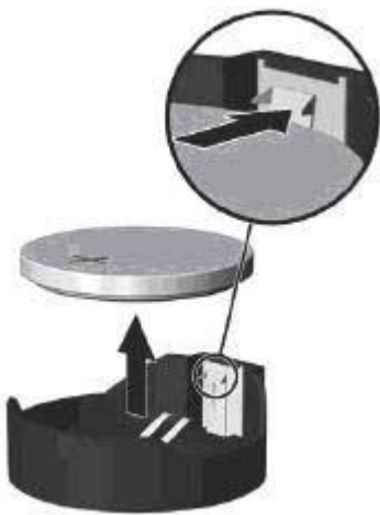
Figure 17 : Type 2 battery holder
