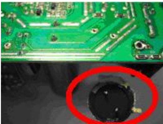
Figure 17 : Type 2 battery holder
