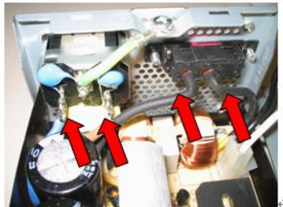
Figure 12: Cut all cables connected to the board
