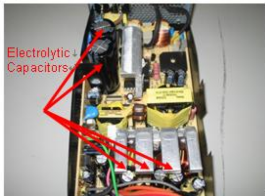
Figure 13 : Electrolytic Capacitors location
