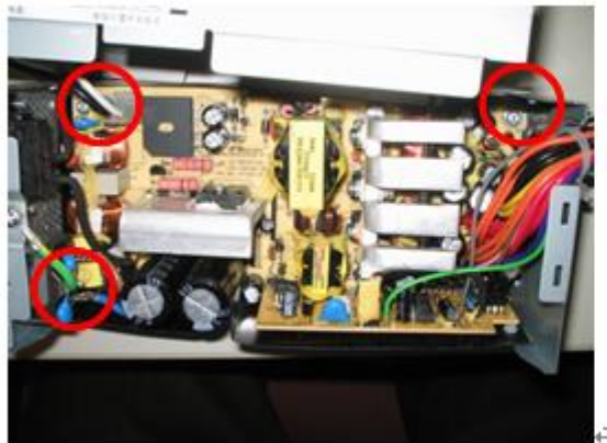
Figure 11: Power supply PCA screw location
