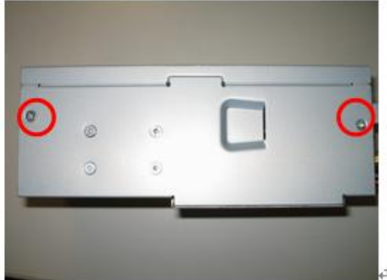
Figure 8: Power supply cover screw locations on the bottom side
