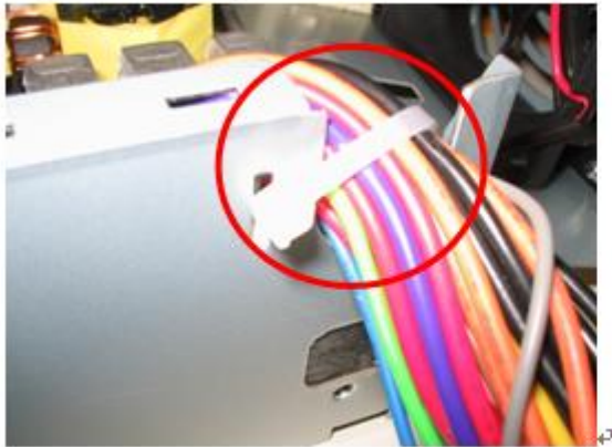
Figure 9: Cut the plastic cable clamp
