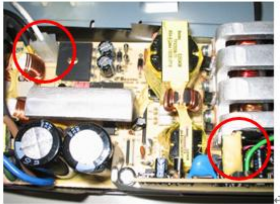
Figure 10: Disconnect two control cables
