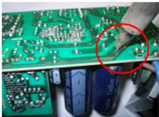
Figure 14 : Heat the solder of Electrolytic Capacitors
