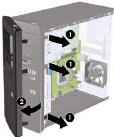
FIGURE 2: Removing the front bezel
