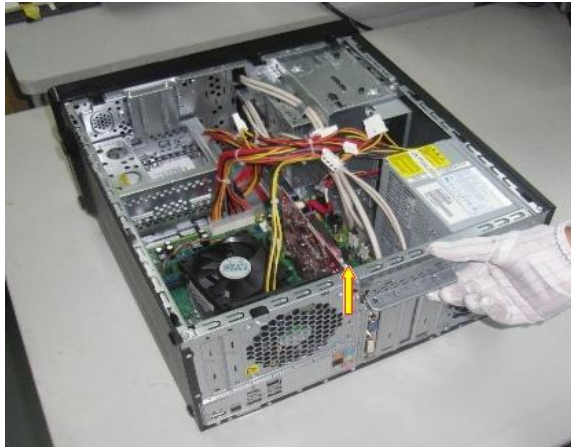
Figure 11 Remove the Graphic card from the board
