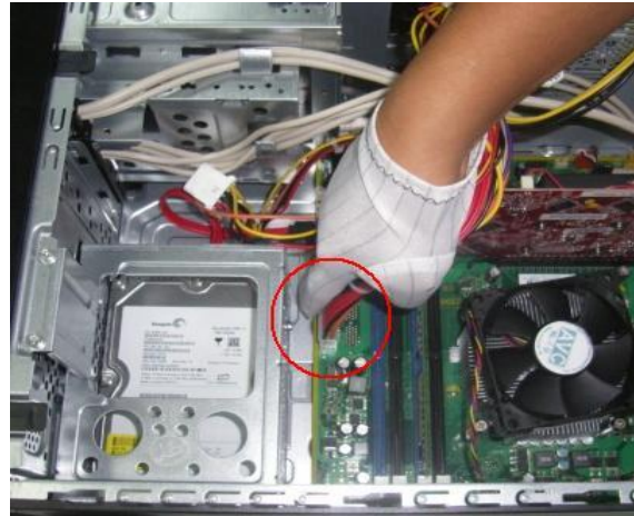
Figure 6 Disconnect the cables from the board
