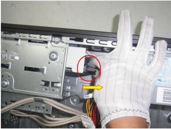
Figure 33 Loose the screws on the ODD cage
