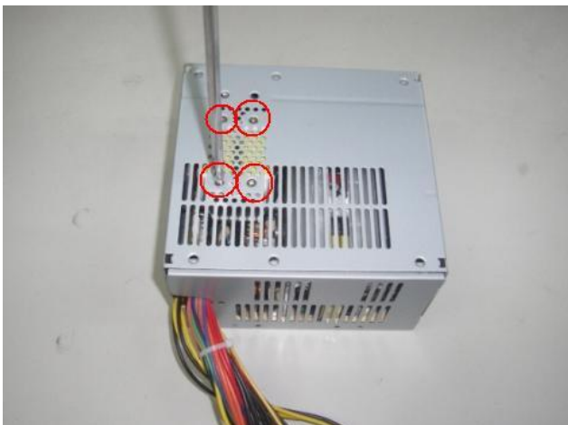
Figure 47 Remove four screws of the PFC module.
