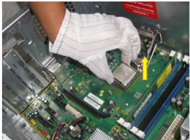
Figure 18 Remove the processor from the socket.
