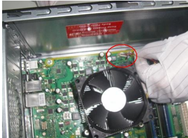
Figure 16 Remove the CPU fan
