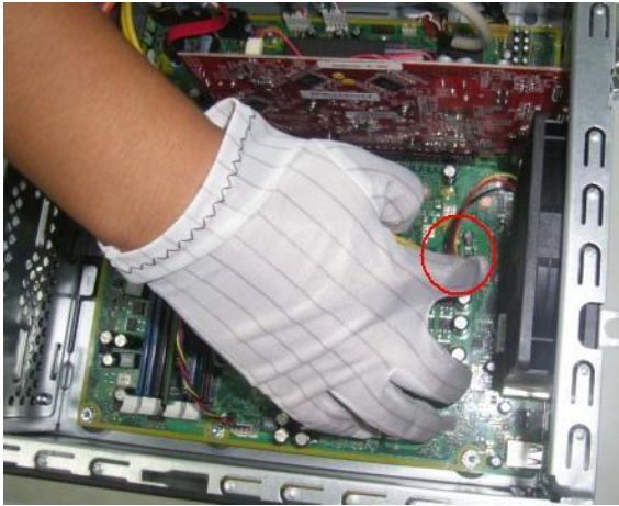
Figure 5 Disconnect the cables from the board
