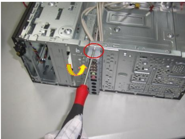
Figure 35 Loose the screw of the front I/O to chassis.
