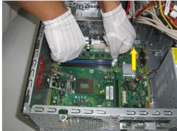
Figure 22 Lift the mainboard from the chassis
