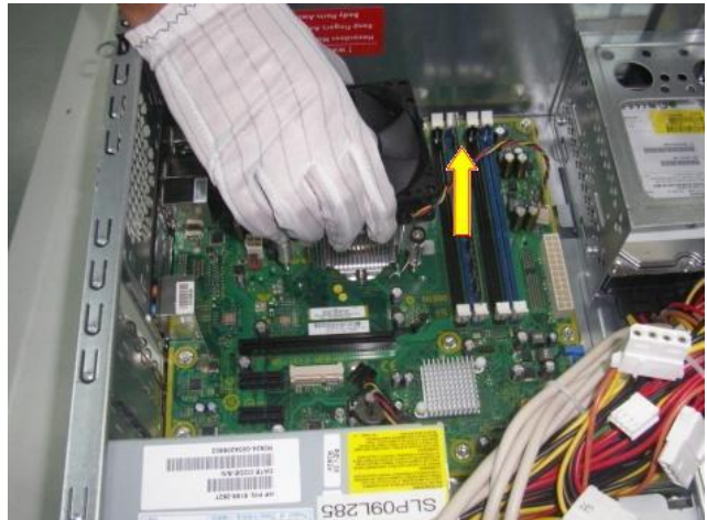
Figure 18 Remove the processor from the socket.
