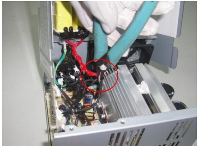
Figure 48 Lift the PFC out of the power supply cage
