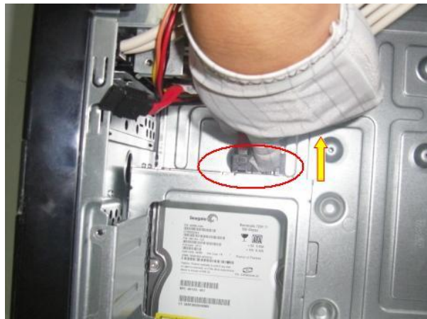
Figure 24 Remove the cables connect to the HDD.
