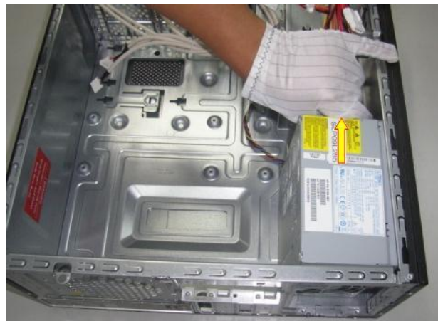
Figure 42 Lift the power supply out of the chassis.
