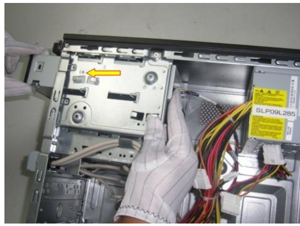
Figure 36 Cut the plastic cable clamp
