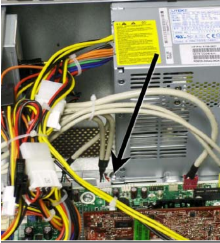
FIGURE 10: POWER SUPPLY: Screw locations
