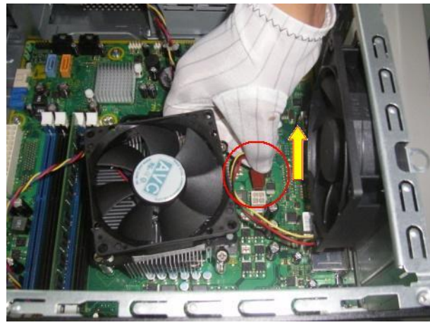
Figure 12 Disconnect the system fan from the board
