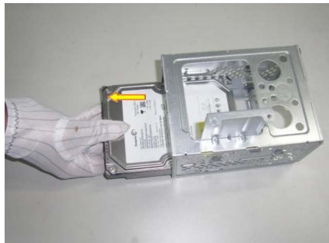
Figure 30 Pull the HDD from the HDD cage
