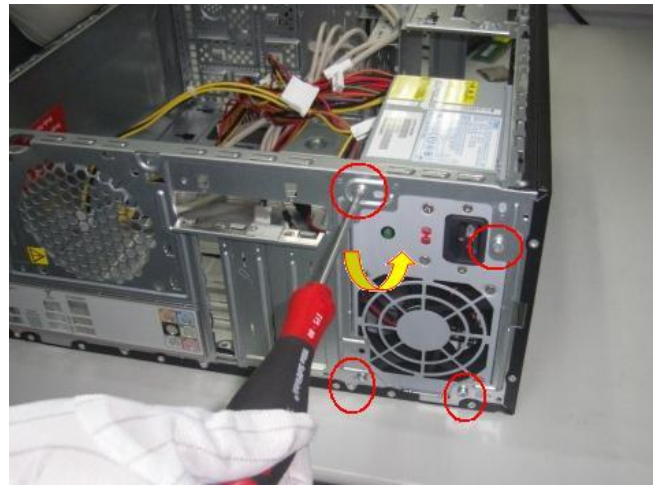
Figure 42 Lift the power supply out of the chassis.
