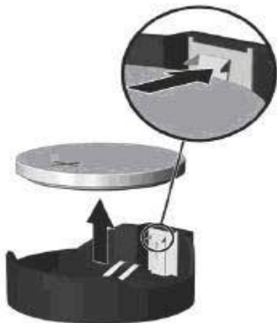
Figure Remove the battery from the system board
