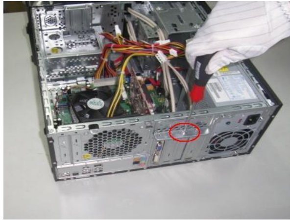
Figure 10 Push the switch of PCI_E slot
