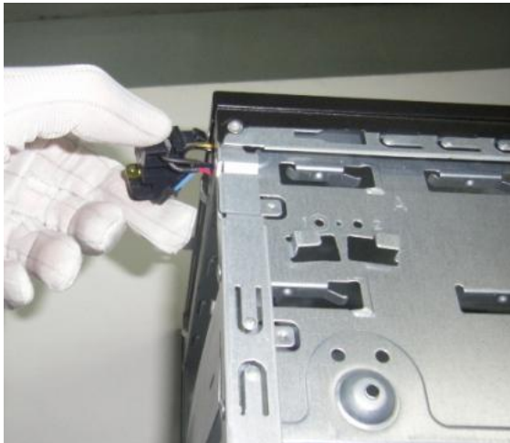
Figure 41 Press the baffle and slide the PSU
