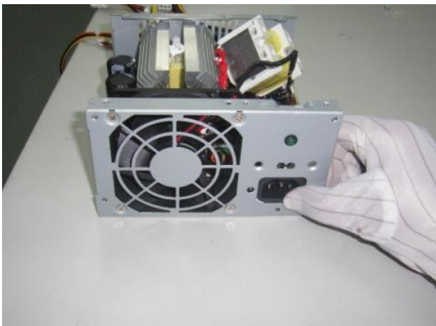
Figure 53 Push the switch and light out of the cage.
