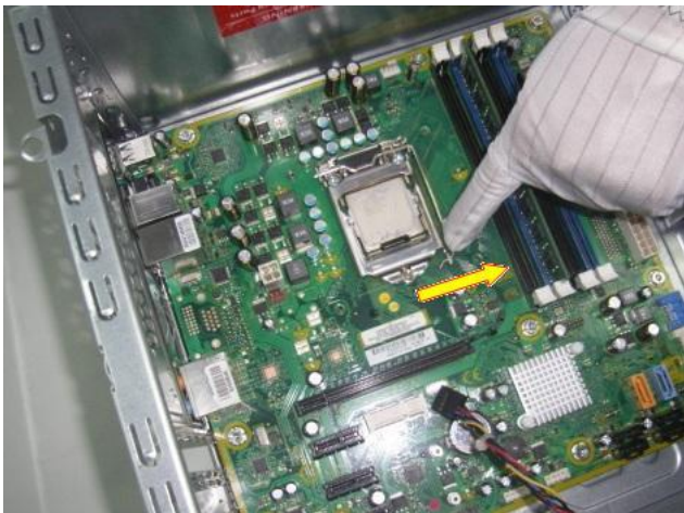
Figure 17 Rotate the handle and open it up
