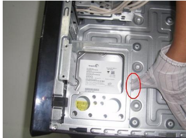
Figure 28 Loose the screws on the side of HDD cage
