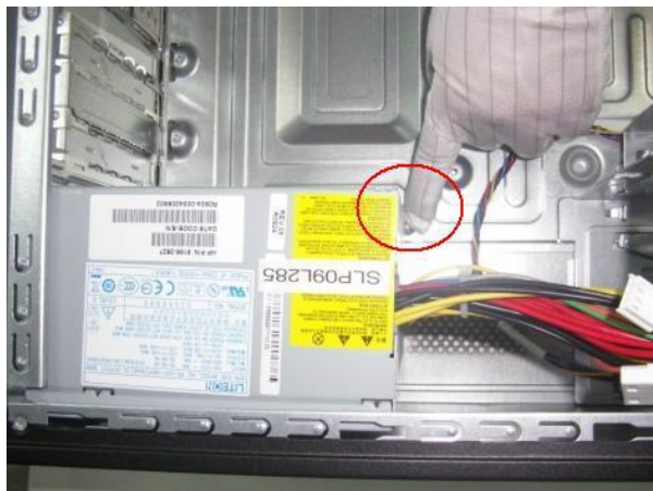
Figure 41 Press the baffle and slide the PSU
