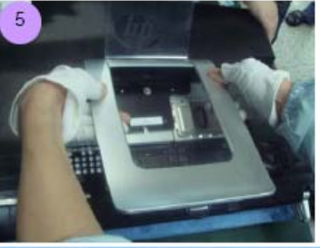
Take the stand out of unit and put it on matrial area
