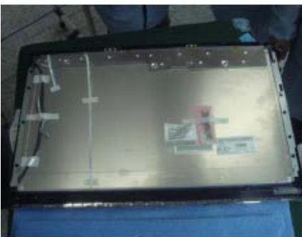
Put the units on inspect jig
