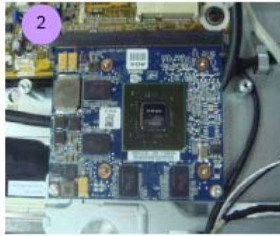
MXM card should lose 2pcs screw to be moved
