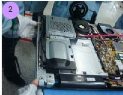
Remove left left side cap from chassis and plug power cable from card
