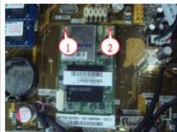
Losse TV card screws and plug out TV card from MB
