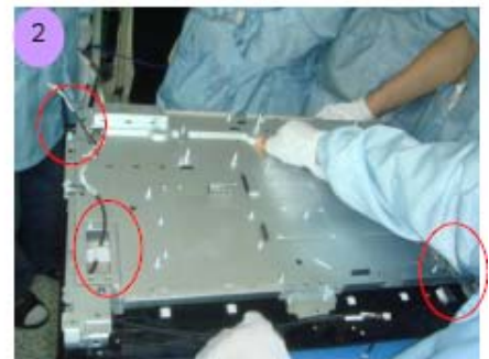
Two operators hold base pan, route panel cable from base pan.
