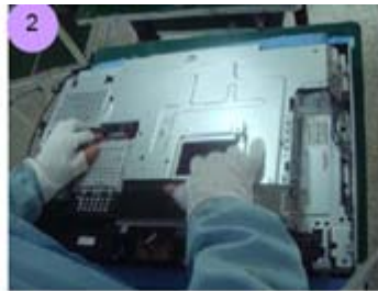
Take rear meter shield from chassis
