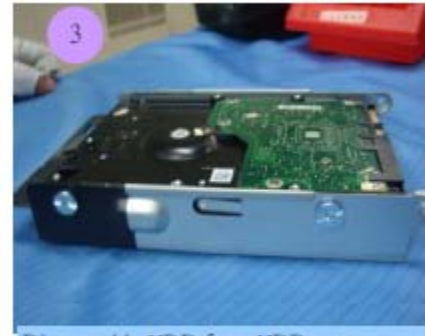
Disassemble HDD from HDD cage
