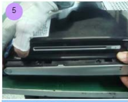
Disassembly ODD plastic cover
