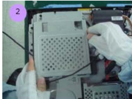
Dis-lock one pcs screw and take ODD from chassis
