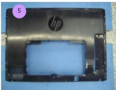
Remove 2 screws in ODD plastic cover and other 3pcs screw on pic shows location
