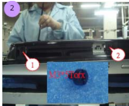
Remove 2 screws in ODD plastic cover and other 3pcs screw on pic shows location
