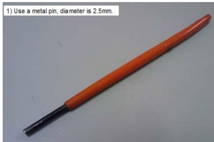
Figure 3 : Remove molded-in NUT from Chin
