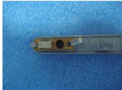
Remove left left side cap from chassis and plug power cable from card
