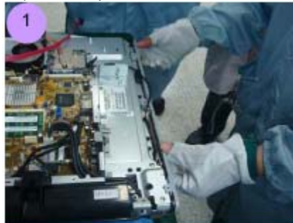
Disassembly right side cap
