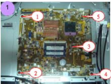
Disassemble 5pcs screws on MB and take MB from chassis
