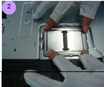
Disassemble DDR shielding
