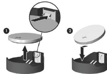
FIGURE 7: Type 3 battery holder
