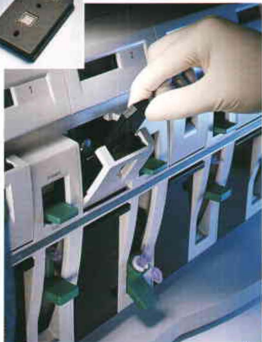
Affymetrix uses HP technology to identify unknown DNA sequences. A researcher inserts a GeneChip probe array—a glass chip, mounted in a cartridge (left inset)—into a Fluidics 400 station (left) for analysis. The whole GeneArray system includes an HP G2500A GeneArray scanner (below), a PC with GeneChip software and the Fluidics 400 station.
