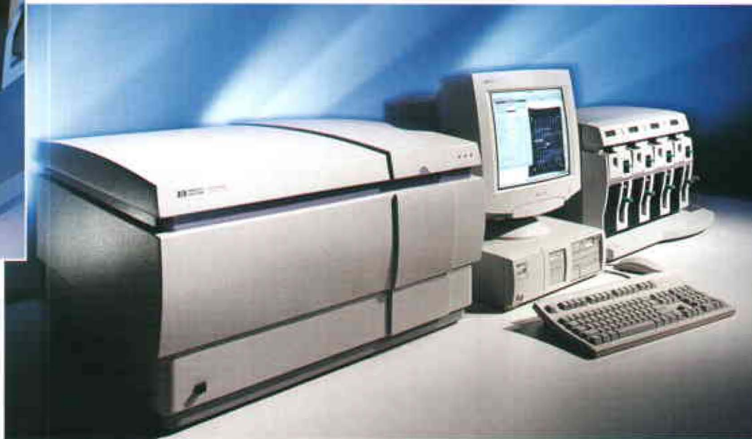
Affymetrix uses HP technology to identify unknown DNA sequences. A researcher inserts a GeneChip probe array—a glass chip, mounted in a cartridge (left inset)—into a Fluidics 400 station (left) for analysis. The whole GeneArray system includes an HP G2500A GeneArray scanner (below), a PC with GeneChip software and the Fluidics 400 station.
