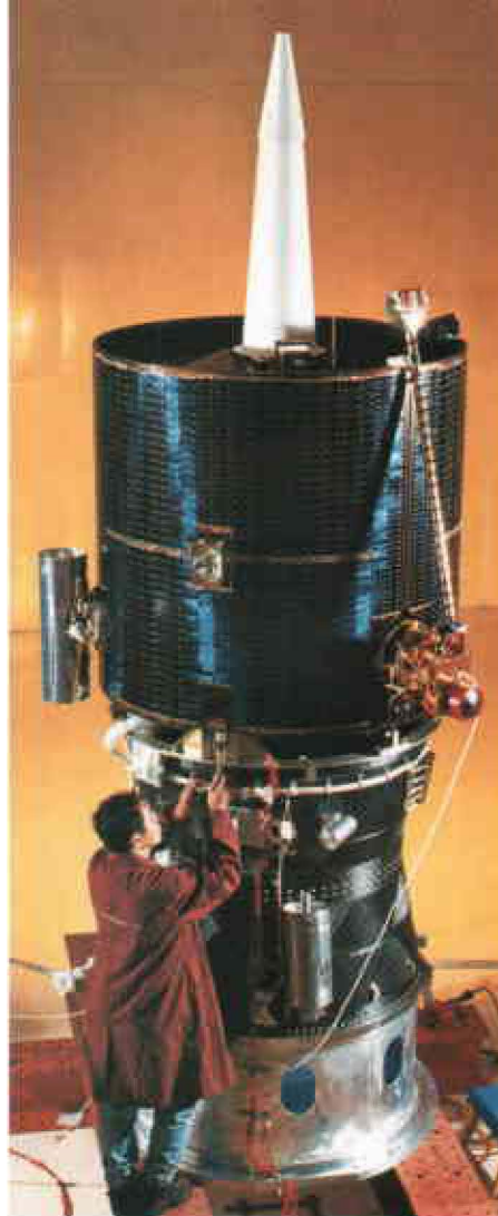
The fully assembled Lunar Prospector sits atop the Trans Lunar Injection stage, which detached about one hour after launch.
