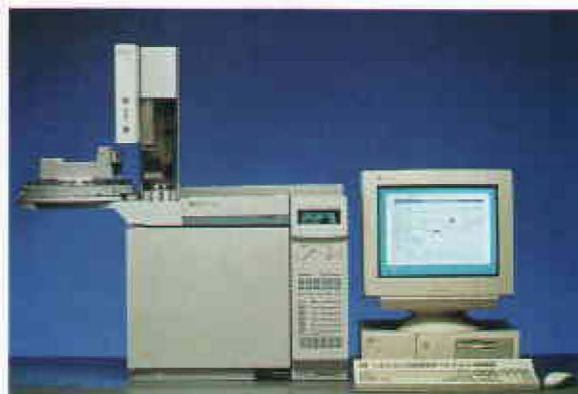
HP 6890 series gas chromatography system has complete electronic control of all gas pressures and flows.
