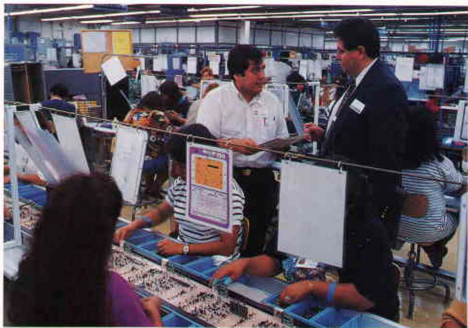
HP spectrum analyzers test TV-top signal converters at Edemsa-Jerrold Communications, where Ramiro Chavez Torres, test-equipment engineering manager, talks with Henry.
