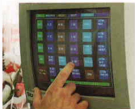
UDF clerks can ring up purchases accurately just by touching the appropriate category on the HP 9000 screen.
