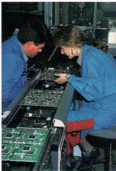
Battista Salvi (left) and Barbara Giroto inspect formatter boards on the Bergamo manufacturing line.
