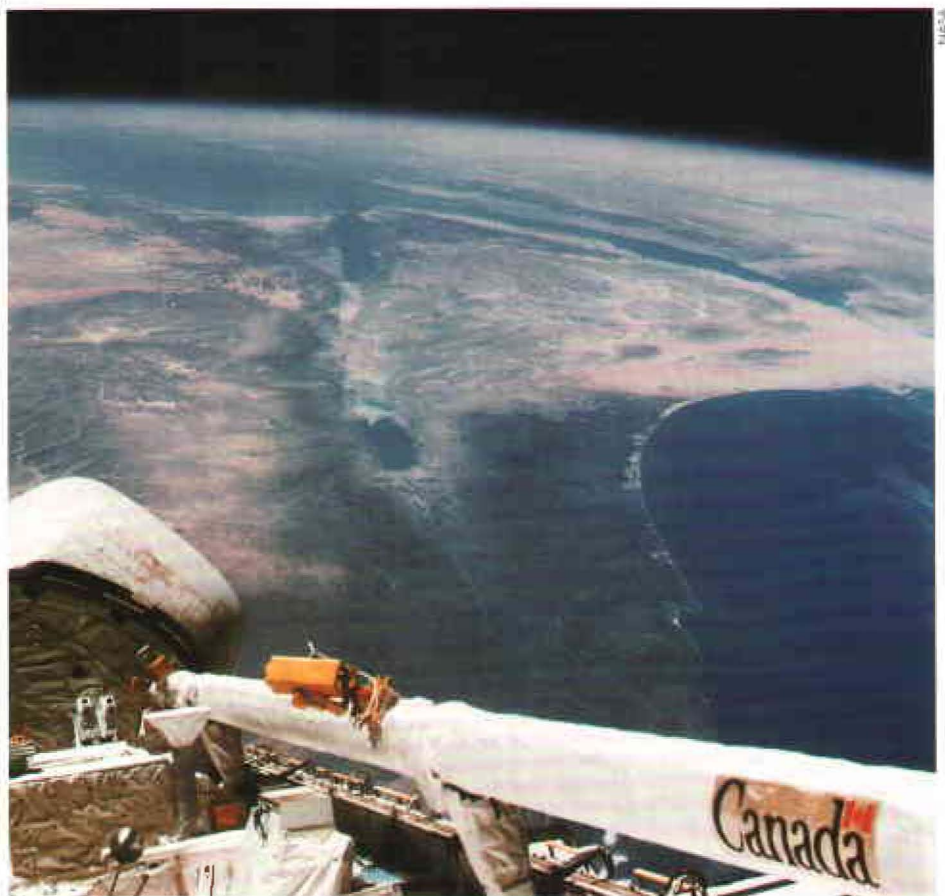
The HP-tested Canadarm, developed by Canada's Spar Aerospace, can deploy or retrieve satellites as large as four 18-wheel trucks in space.
