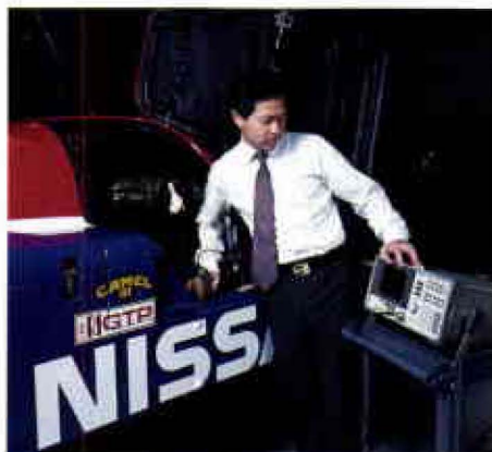
HP engineer Bert Dare uses a probe to test for electromagnetic interference.
