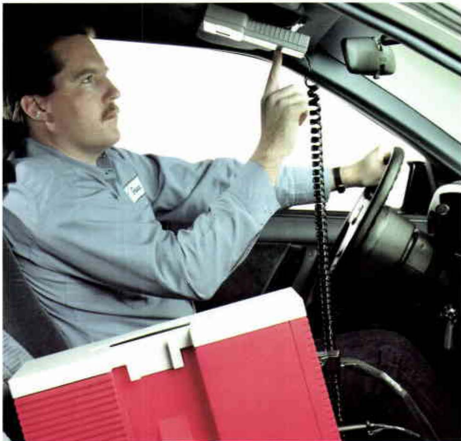
Technicians can detect some automotive problems by using a Portable Vehicle Analyzer during road tests. Information from the unit can be transferred directly to an SBDS computer.
