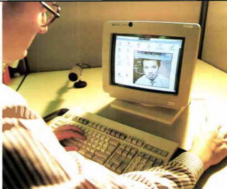
Stephen Gale and Colin Baker (on screen) can see and hear each other while they share data on this prototype system developed at HP Labs Bristol.
