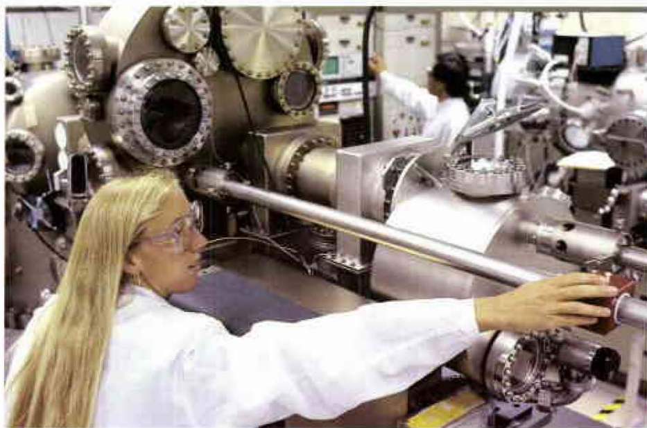
HP Labs researcher Alice Fischer-Colbrie uses a molecular-beam epitaxy machine to deposit gallium arsenide—atomic layer by atomic layer—to develop transistors, integrated circuits and optical devices.
