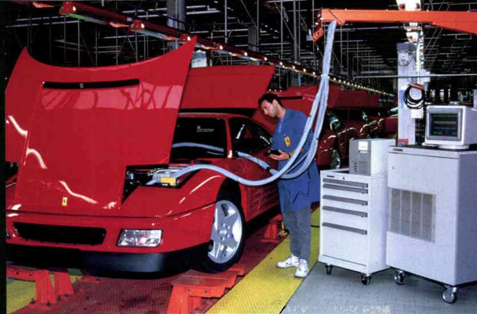
Equipment from HP's Advanced Manufacturing Systems Operation tests the electrical system of the Ferrari 348 at four of the 20 work sites.
