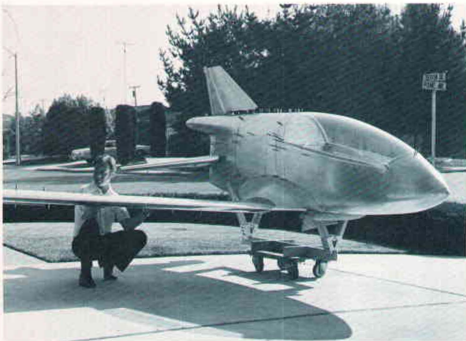
The BD-5, a single-place kit airplane with retractable landing gear and a "pusher" prop looks a bit like a rocket plane somehow mislaid on a suburban street as Jim Hergert fits one of the wings. He's building the tiny aircraft in his one-car garage—and still has room for the car!
