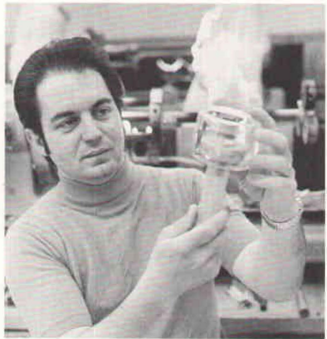
Holding what appears to be an Olympic torch is Jerry Black who heads the glass-blowing department. Actually the glass item is a laser envelope produced at Santa Clara for the HP laser interferometer (the flame is safely in the background). The department produces a variety of glass products including very sophisticated work for HP rubidium standards.
