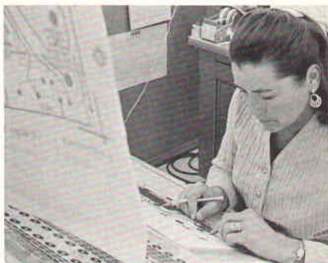
Versatile computational abilities of new counter are based in large part on extensive use of printed circuits and IC's. Here Gladys Kinney works on artwork for new PC board.
