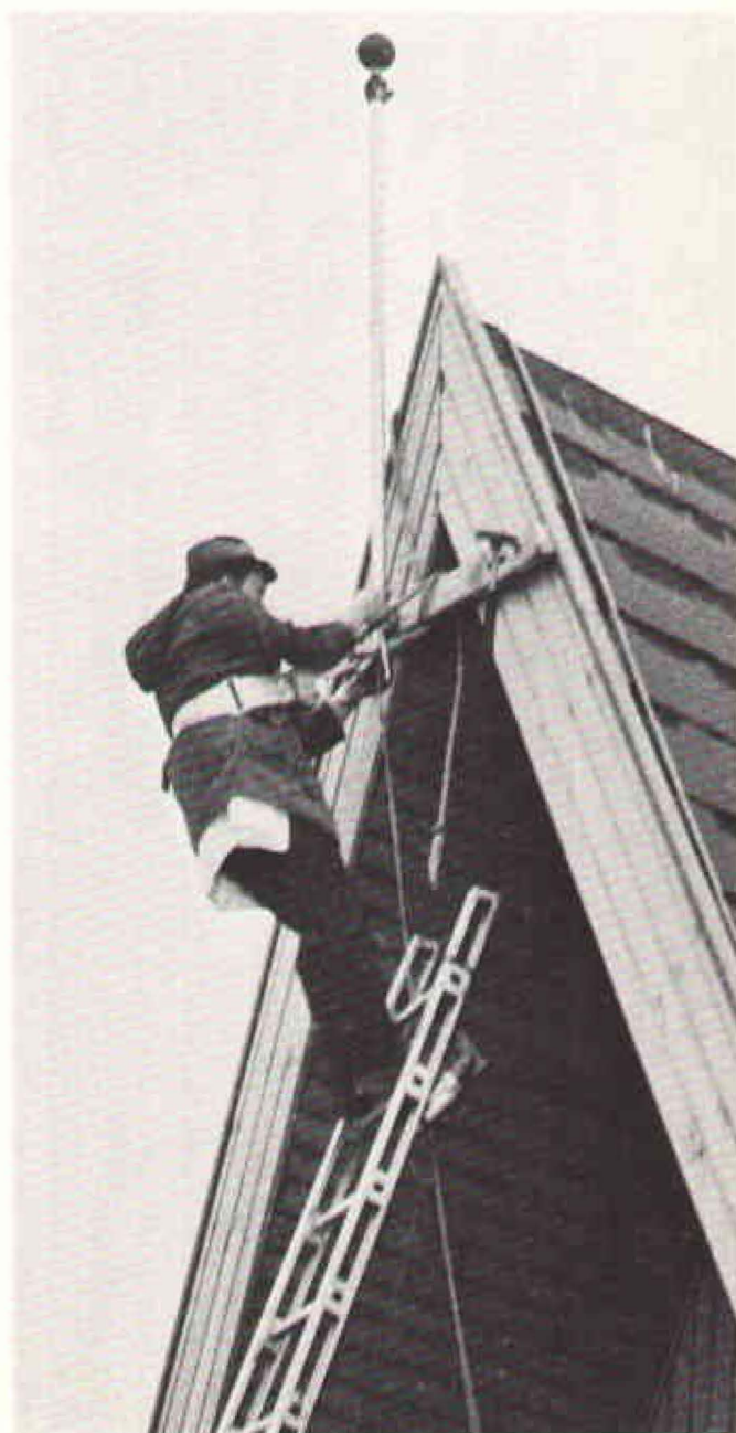
Looking something like a short flagpole, outdoor microphone is attached to roof, below, of a noise monitoring terminal building. Inside, Helmut Finkh, R and D project leader at left, and Rainer D'Arcy, acoustics product manager, conduct final testing at one of the seven terminals around airport.
