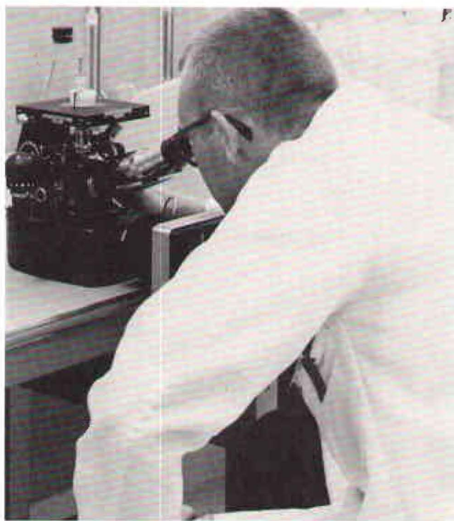
Loveland's Larry Huston checks a cross section of a multi-layer printed circuit board using metallurgical microscope with attached camera. He looks for such things as proper alignment, bonding, and electroplating of the through holes for connections to the inner circuits.
