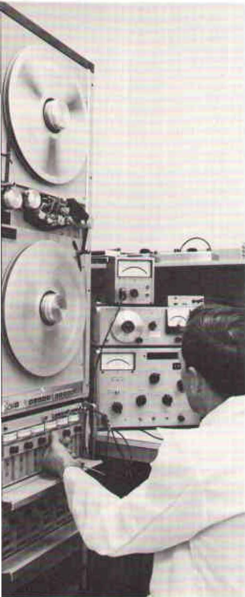
Bill McPeak, Paeco test technician, tests new 1.5 mc tape head with new Microwave tape transport. Tape head must be within 3 microinches of flatness and feature a gap less than 30 microinches across—one-hundredth the diameter of a human hair.
