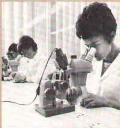
Assembling tiny tape-head parts under microscope are, from right: Jacqueline Vuille, Priscilla Bumbaca, Yuri Katai, Dee Carver.
