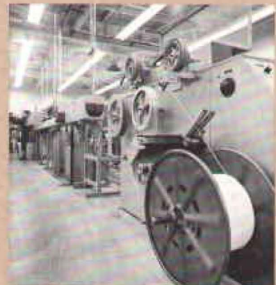
Coating wire with extruded plastic is one phase in the production of Paeco electronic cable. Tending the extruder is Richard Pahler.
