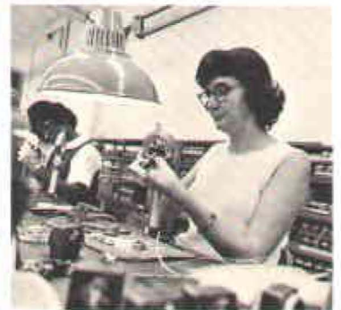
A coil to servo motor is wound by Dorothy Alexander.
