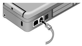
3. Plug the other end of the cord into a telephone jack. If the plug on the phone cord doesn't fit the jack, you may need to use an adapter.
