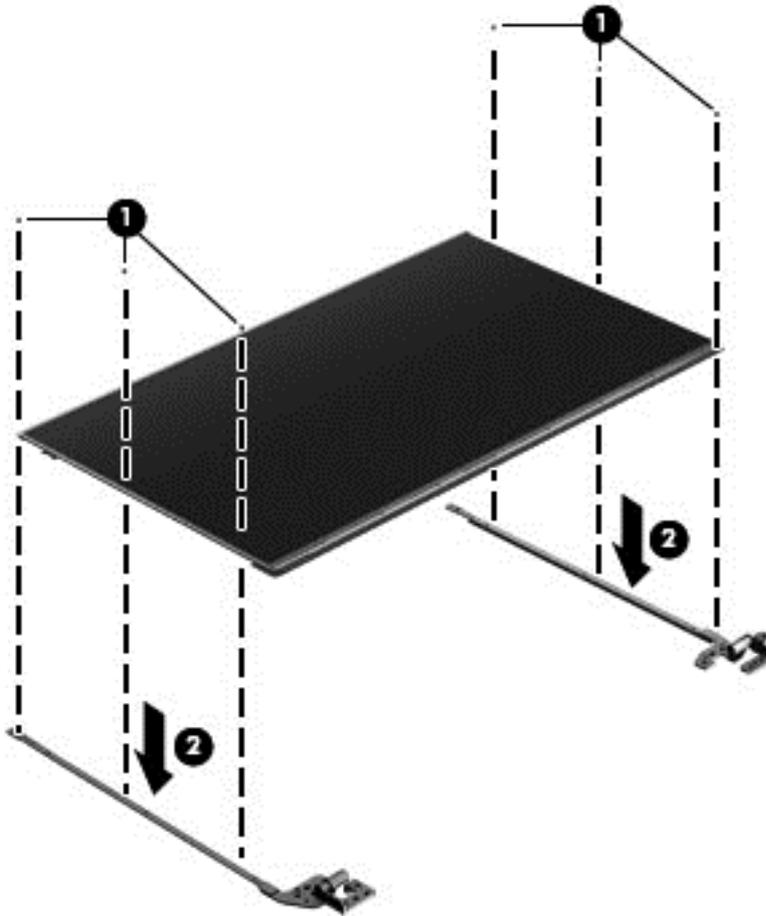
Reverse this procedure to reassemble and install the display assembly.
