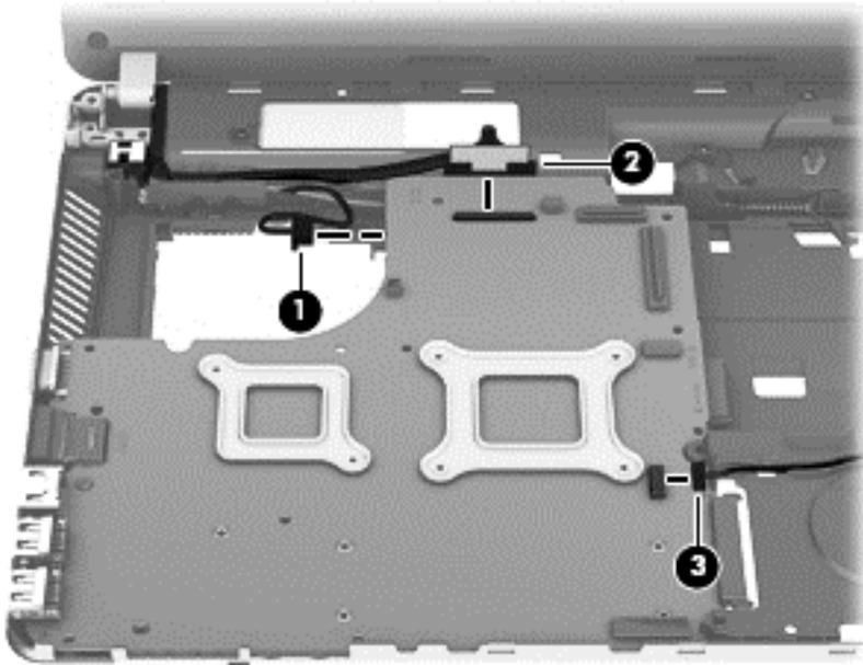
3. Remove the two Phillips PM2.5×4.0 screws (1) that secure the system board then, lift the system board (2) to access the battery cable connector.
