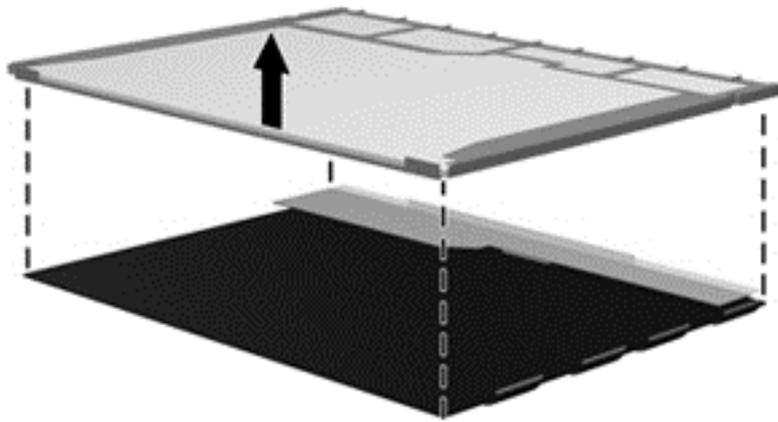
24. Recycle the LCD panel and backlight.
