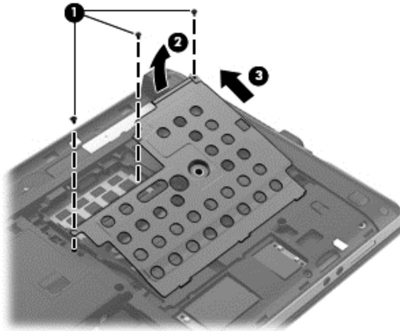
Reverse this procedure to install the metal heat shield.
