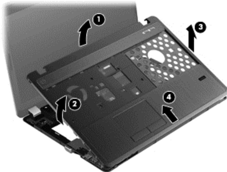
9. With the top cover at an angle (1), disconnect the audio board cable (2) from the system board, and then remove the top cover from the computer .
