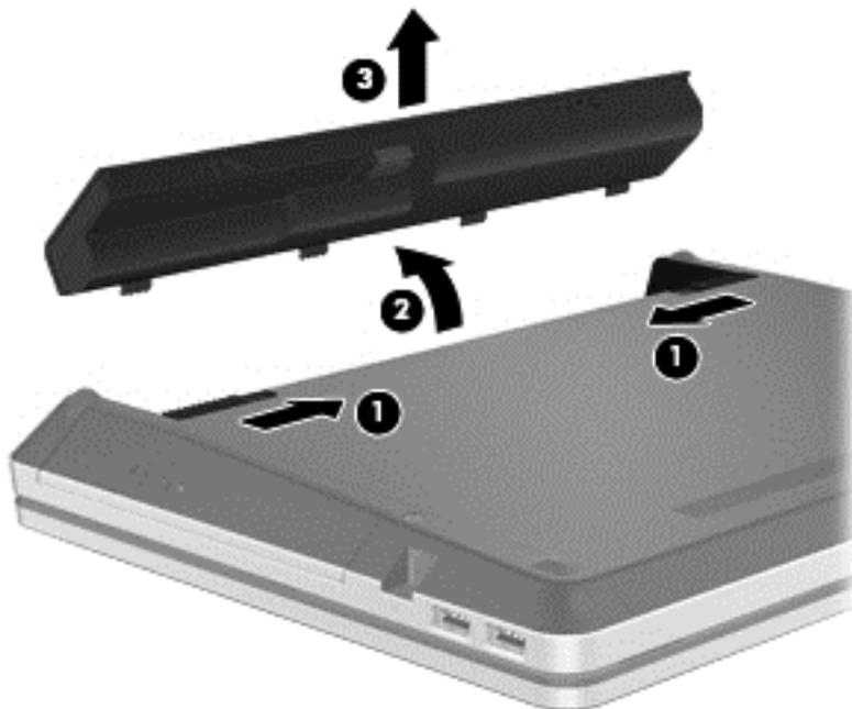
Install the battery by inserting it into the battery bay until you hear a click.
