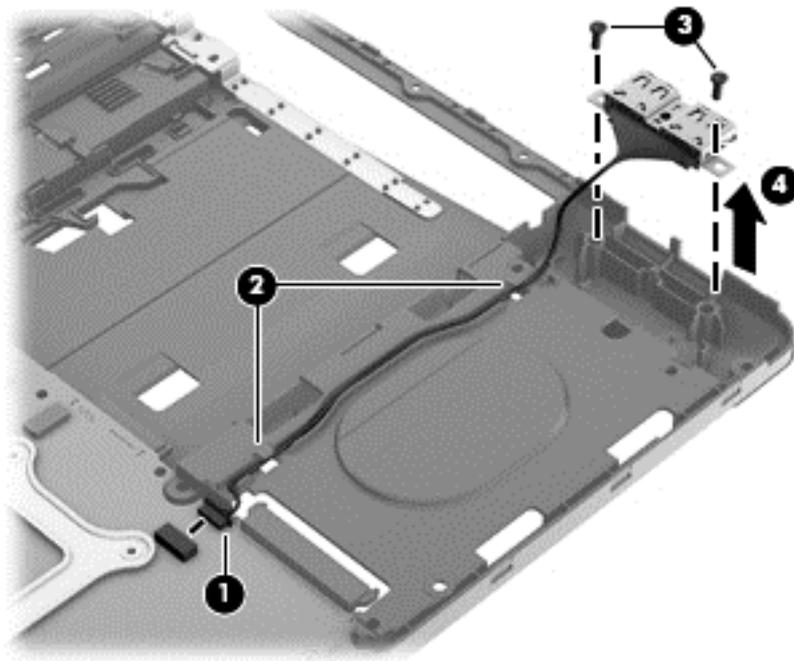
Reverse this procedure to install the USB module.
