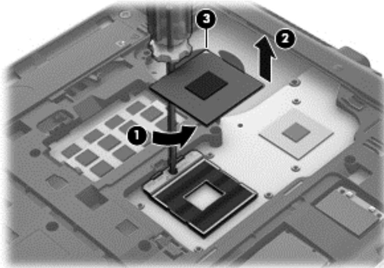
Reverse this procedure to install the processor.
