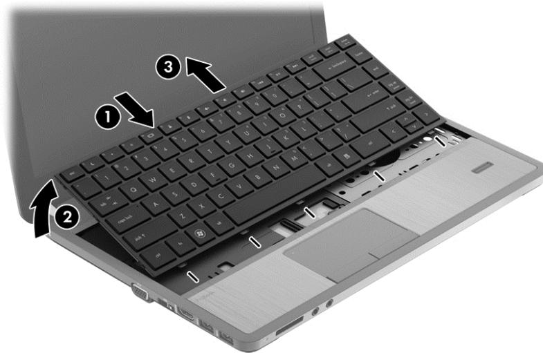
7. Rotate the keyboard until it rests on the palm rest (1).
