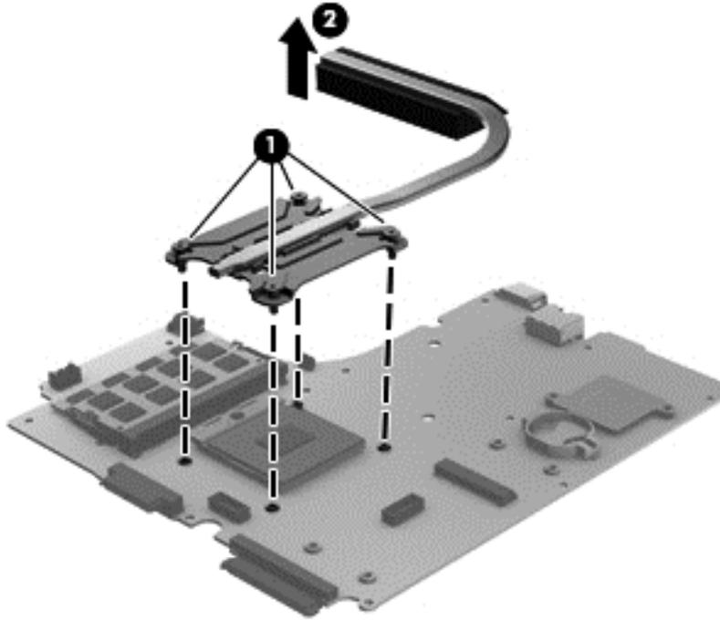
**NOTE:** For discrete models, thoroughly clean thermal material from the surfaces of the system board components (1) and (3) and the heat sink (2) and (4) each time you remove the heat sink. All heat sink and processor spare part kits include thermal material.
