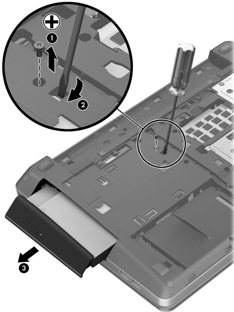
5. If it is necessary to replace the optical drive bracket, position the optical drive with the rear toward you.
