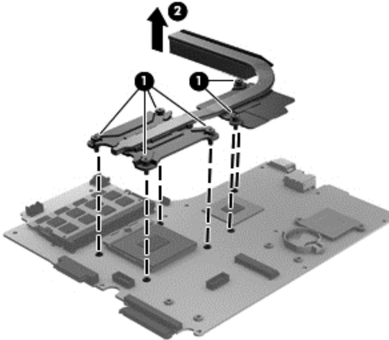
Remove the UMA heat sink.
