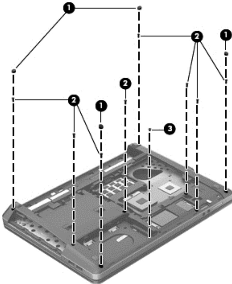
3. Remove the following screws that secure the top cover to the computer:
