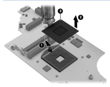
Reverse this procedure to install the processor.
