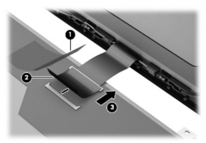
**d.** Remove the display panel. The display panel is available using spare part numbers 653378-001 (for use with computer models equipped with a 15.6-in, FHD, LED, AntiGlare
