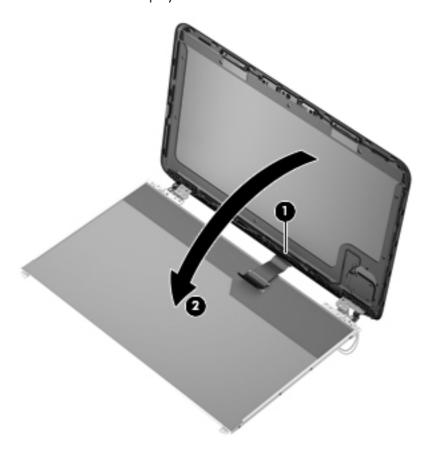
c. Release the adhesive strips (1) and (2) that secure the display panel cable to the display panel, and then disconnect the display panel cable (3) from the display panel.
