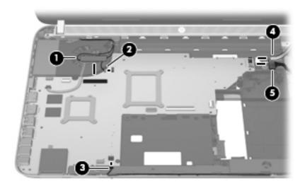
7. Remove the Phillips PM2.5×4.0 screw (1) and the two Phillips PM2.5×5.0 screws (2) that secure the system board to the base enclosure.
