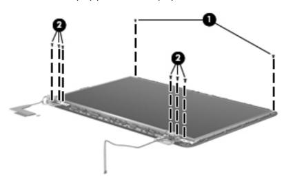
**b.** Lift the top edge of the display panel (1), and then swing it forward (2) until it rests upside down in front of the display enclosure.
