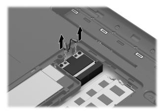
2. Remove the two Phillips PM2.0×4.0 screws that secure the WLAN module to the system board. (The WLAN module tilts up.)
