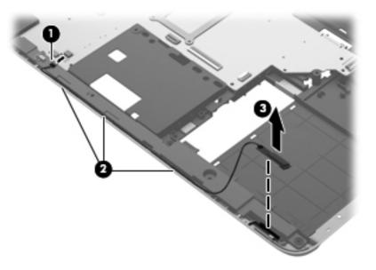
4. Remove the Bluetooth module and the Bluetooth module cable.
