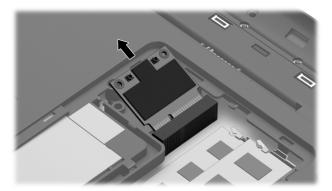
NOTE: If the WLAN antennas are not connected to the terminals on the WLAN module, the protective sleeves must be installed on the antenna connectors, as shown in the following illustration.
