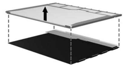
**24.** Recycle the LCD panel and backlight.
