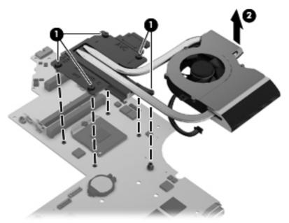
NOTE: The following illustration shows the fan/heat sink assembly being removed from a computer model equipped with an Intel processor and a graphics subsystem with discrete memory. A computer model equipped with an Intel processor and a graphics subsystem with UMA memory has only four screws.
