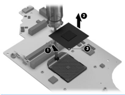
NOTE: The following illustration shows the processor removal process on a computer model equipped with an Intel processor.
