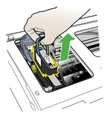
5. Before installing a printhead, shake the printhead up and down at least six times while the printhead is still in its packaging.
