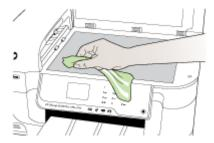
△ **CAUTION:** Use only glass cleaner to clean the scanner glass. Avoid cleaners that contain abrasives, acetone, benzene, and carbon tetrachloride, all of which can damage the scanner glass. Avoid isopropyl alcohol because it can leave streaks on the glass.
