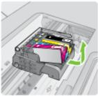
4. Lift the latch handle on the print carriage.
