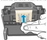
**b**. Use a fresh, lightly dampened, lint-free cloth to wipe any accumulated ink and debris from the edge between the nozzles and the contacts.
