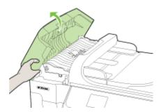
**3.** Continue lifting the automatic document feeder cover to the vertical position.
