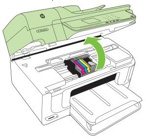
The print carriage moves to the center of the printer.
