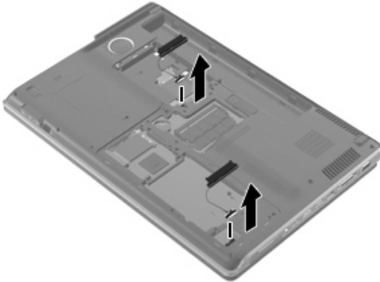
3. Remove the two Phillips PM2.5×5.0 screws (1) that secure the system board to the base enclosure.
