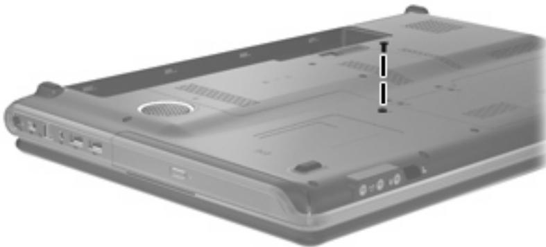
**Where used:** One screw that secures the optical drive to the computer
