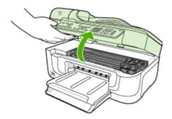
**3.** Remove the print cartridges from their slots by grasping each between your thumb and forefinger and pulling it firmly toward you.
