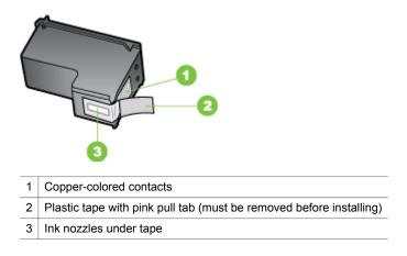
Hold the print cartridges by their black plastic sides, with the label on top. Do not touch the copper-colored contacts or the ink nozzles.
