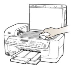
△ CAUTION: Use only glass cleaner to clean the scanner glass. Avoid cleaners that contain abrasives, acetone, benzene, and carbon tetrachloride, all of which can damage the scanner glass. Avoid isopropyl alcohol because it can leave streaks on the glass.
