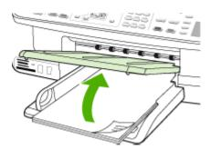
2. Insert the media print-side down along the right of the tray. Make sure the stack of media aligns with the right and back edges of the tray, and does not exceed the line marking in the tray.
