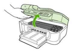
**3.** Wait until the print carriage is idle and silent, and then lightly press down on a print cartridge to release it.
