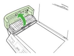
4. Lift the automatic document feeder mechanism.
