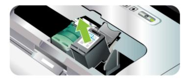
4. Insert the new print cartridge into its cradle compartment at the same angle at which you removed the old print cartridge. Check the symbol on the latch against the symbol on the print cartridge to make sure you are inserting the correct print cartridge.
