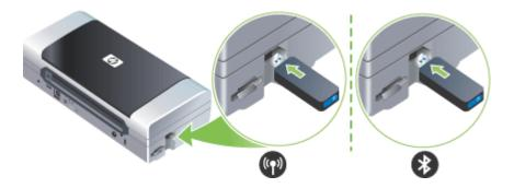
Insert the HP 802.11 or Bluetooth wireless USB accessory into the slot.
