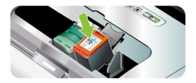
Close the print cartridge latch. If the cartridge is inserted correctly, closing the latch gently pushes the cartridge into its cradle compartment. Press the latch to make sure it is seated flat on the cartridge.
