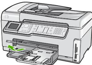
2. Insert the stack of photo paper into the photo tray with the short edge forward and the glossy side down. Slide the stack of photo paper forward until it stops.
