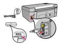
**IMPORTANT:** If your printer has a USB port on the front, do not attach the printer adapter to it. Use the back USB port.
