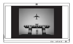
□ Fill to Screen — This display format adjusts the horizontal and vertical size of the image to fill the screen. Aspect ratio is not preserved, so the image appears stretched. There are no black borders at the edge of the display.
