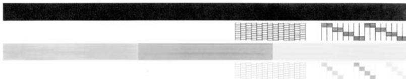
3. Make sure the test patterns show a complete grid and that the thick colors lines are complete.
