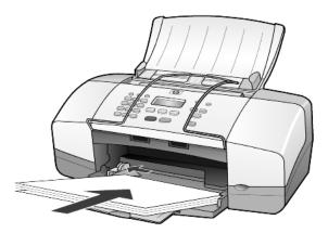
5 Slide the paper-width guide in until it stops at the edge of the paper. Make sure that the paper stack lies flat in the paper tray and fits under the tab of the paper-width guide.
