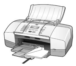
3 Adjust the paper-width guide against the envelope until it stops. Be careful not to bend the envelope.
