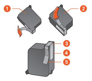
1. black cartridge 2. tri-color cartridge 3. ink nozzles 4. copper contacts-do not touch or remove the copper contacts 5. protective vinyl tape-remove only the protective vinyl tape
