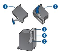
black print cartridge 2. tri-color print cartridge 3. ink nozzles 4. copper contacts
